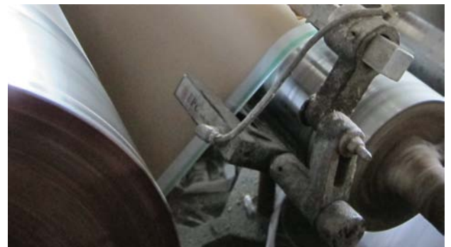
Infrared Sensor DS-26L is used on Inner Edge Position Control
