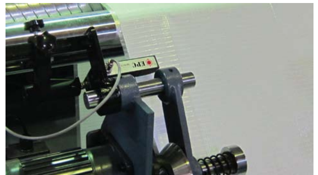
Infrared Sensor DS-26L is used on a Extrusion Laminator
